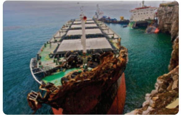
MV Fedra broken in half adjacent to the Europa Point lighthouse, Gibraltar. (Copyright Stephen Bennett and licensed for reuse under a Creative Commons Licence)
