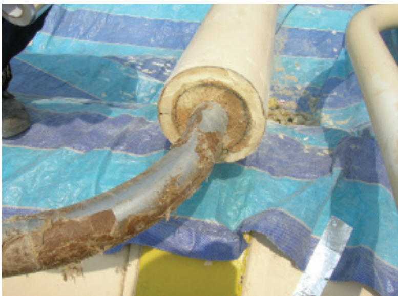
Cryogenic insulation on board an LNG ship – commonly blown using CFCs (Robin Townsend).
