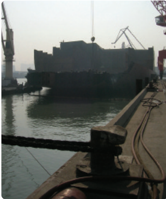
A vessel being recycled alongside: the engine room is ballasted clear of the water, cranes are removing machinery, and an oil spill boom is visible (Robin Townsend).
