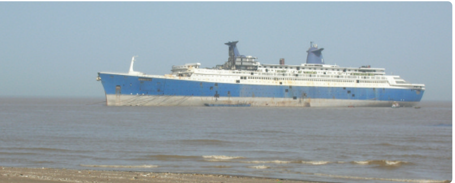
Blue Lady on the beach at Alang. Note the missing forward superstructure, and the holes cut for light and ventilation. (Robin Townsend)
