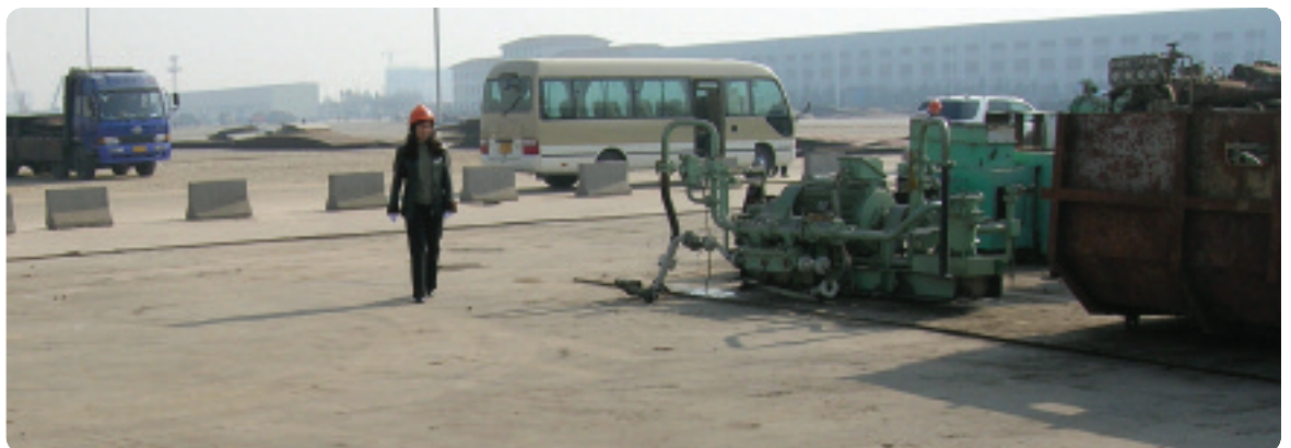
An oily equipment/oily block treatment/cleaning area. Note the steel plate which provides further protection to the concrete floor. This area is exceptionally clean despite constant use, due to the yard's commitment to quality (Robin Townsend).
